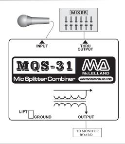
Thank you for your choice of the MQS-31 Mic Splitter. This unit was designed to produce two balanced XLR signals, one direct one transformer isolated, from one single XLR input signal. A ground lift switch has been provided to eliminate some cases of hum caused by ground loops.
